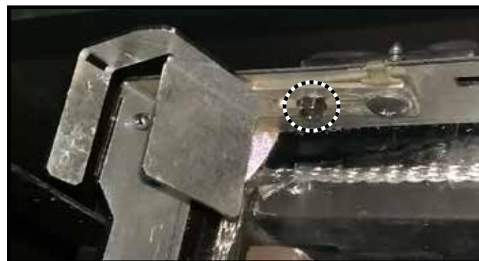
Figure 6. Shipping Location of Refractory Brackets
