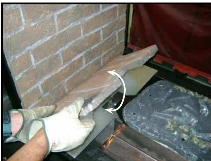
Figure 3. Positioning Inner Bottom Refractory
